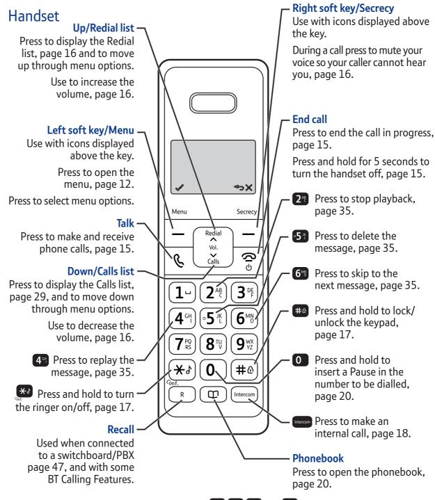
The answer machine handset controls on buttons 2\* 4\* 5\* and 6\* will only work when a message is being played on the handset, page 35.
